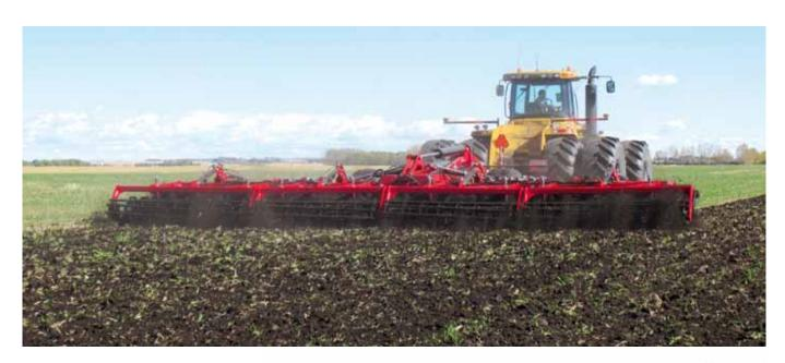
The working widths of 10 and 12 meters of the DBMxT are solved using the G-frame, which offers full user comfort in the standard version. Adjusting the working depth is fully hydraulic with position locks using hydroclips. The machine can be equipped with a flexible skid against the supporting roller and rod grate between the first and second series of discs. Both of these additional working sections can be easily removed from service.
