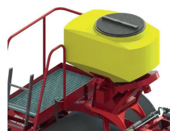
SEEDING ATTACHMENT hopper capacity 200-500 l
